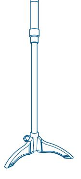
3. Attach the 3" PVC and the two smaller 6" PVC pieces to the Tee fitting as shown.
